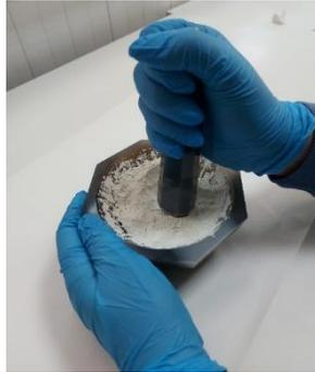
LLZO powder was milled in a mortar for 6 hours.
