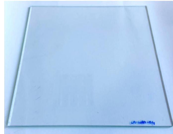
LLZO was deposited on top of the 15 cm x 15 cm SLG substrate.
