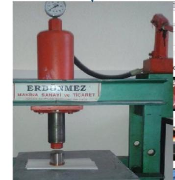
LLZO powder was pressed onto a copper plate under 80 bar pressure.
