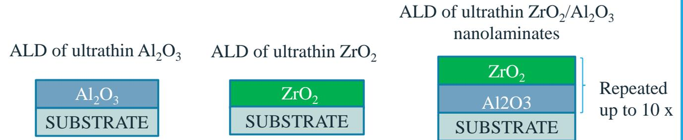
**ALD precursors:** for ALD of  $\text{Al}_2\text{O}_3$  - TMAI,  $\text{H}_2\text{O}$  and TMAI,  $\text{O}_3$
