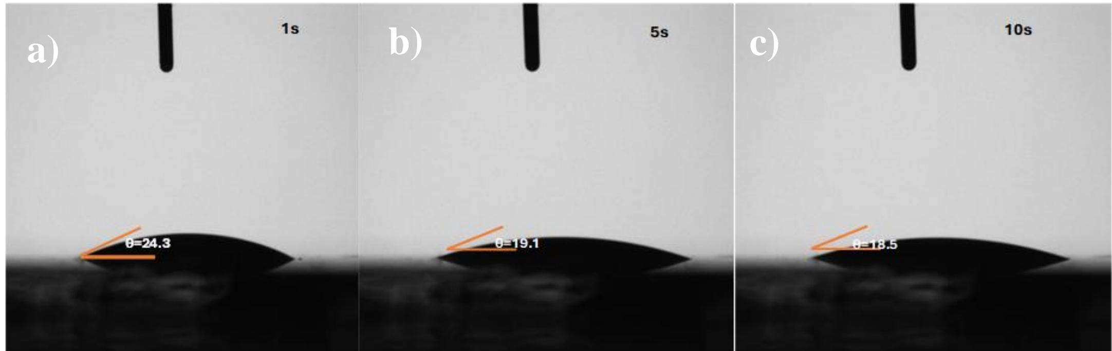
Contact angle images of Ti/LCO thin film samples **a)**  $\theta = 24.3^\circ$ , **b)**  $\theta = 19.1^\circ$ , **c)**  $\theta = 18.5^\circ$
