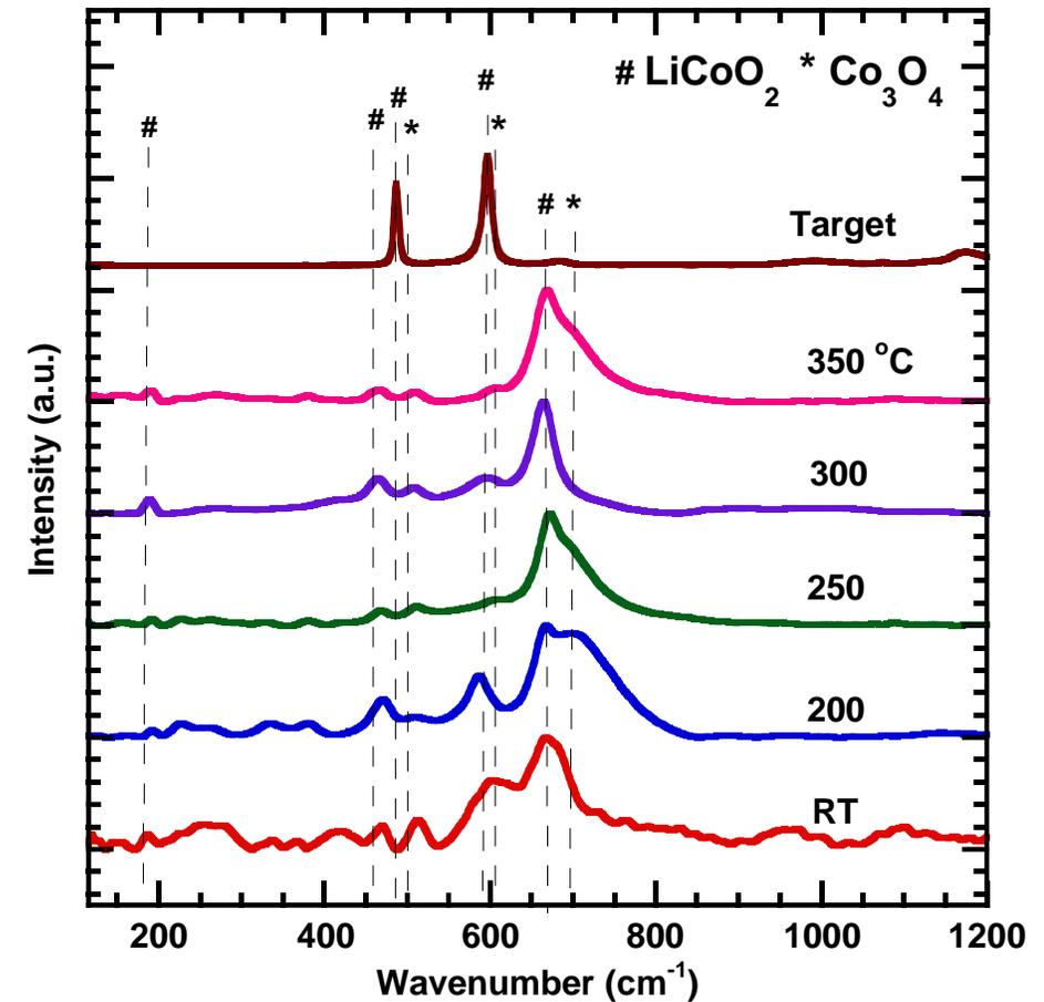
Raman results of LCO target and LCO thin films grown at different substrate temperatures.
