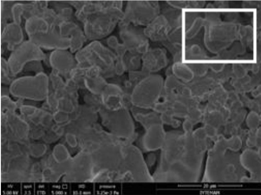
Deformed fragments observed in the SEM image of the LLZO target with size of 20 μm.
