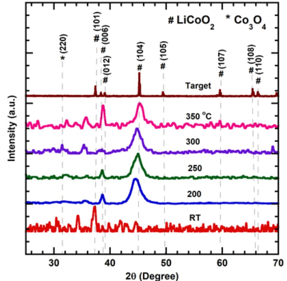
XRD results of LCO target and LCO thin films grown at different substrate temperatures.
