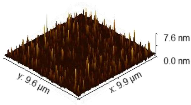
2 nm ZrO<sub>2</sub>/Si - RMS roughness (Sq) = 436.9 pm
