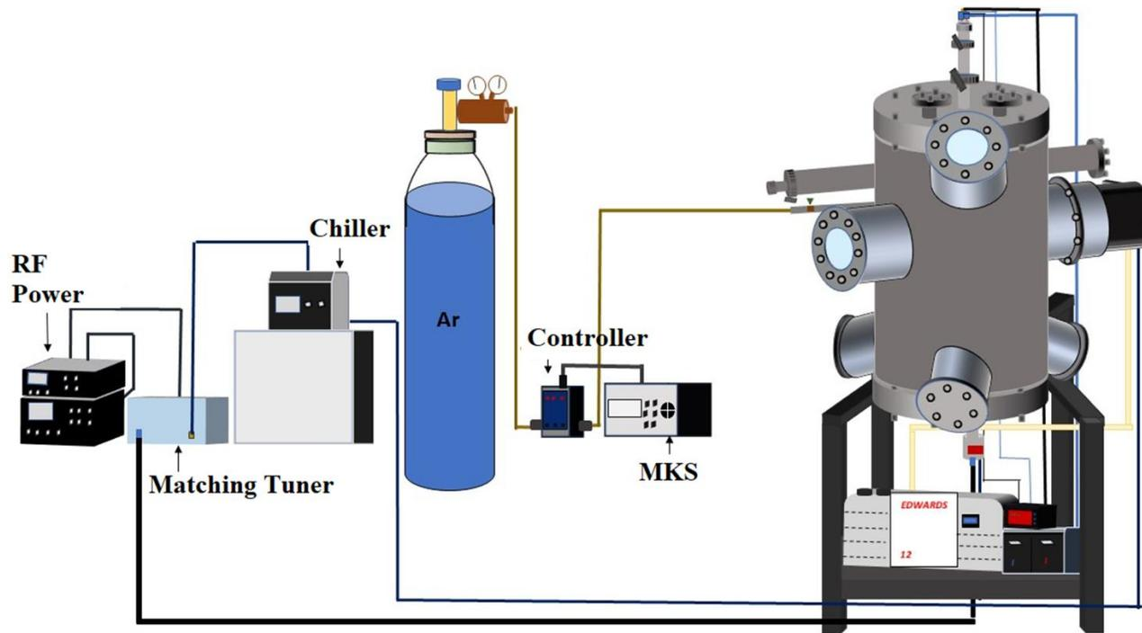
Schematic of magnetron sputtering vacuum chamber
