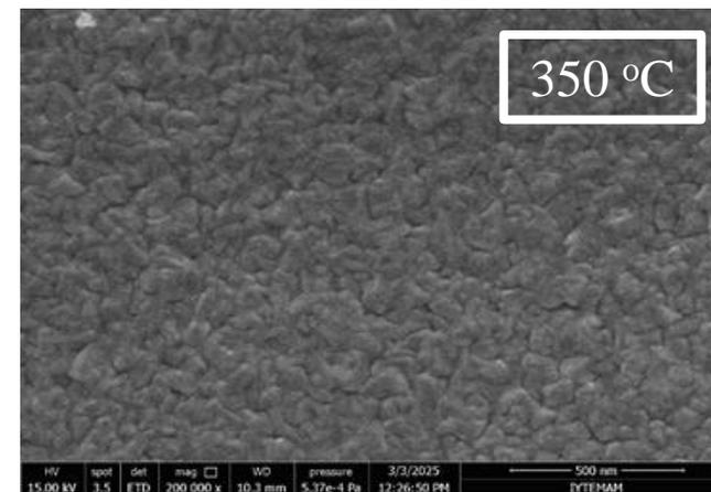
SEM images of LCO thin films grown at different substrate temperatures
