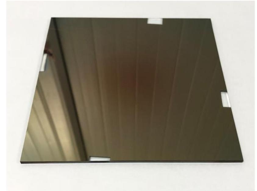
SLG/Ti/LCO thin film deposited on 15 cm x 15 cm glass substrate
