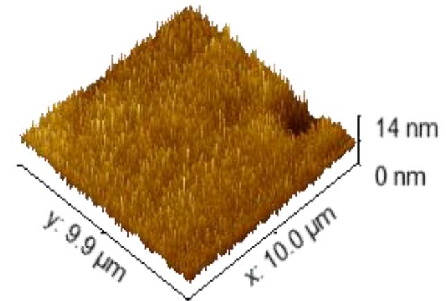
10 x (2 nm ZrO<sub>2</sub>/2 nm Al<sub>2</sub>O<sub>3</sub>) / Si
