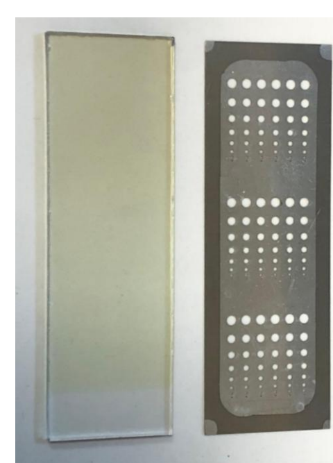
Sample of LLZO grown on ITO coated (contact layer) substrate and the mask
