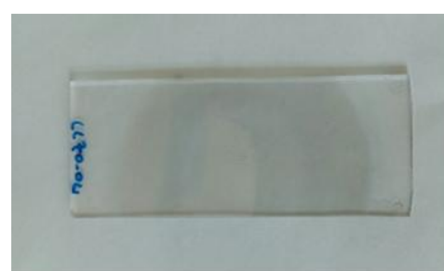
LLZO thin film deposited using 83 W RF Power for 60 minutes
