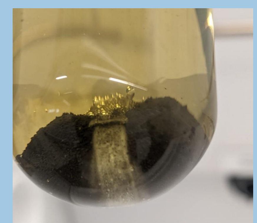
Photograph: metallic cobalt particles amassed around poles of magnetic stirring bar
